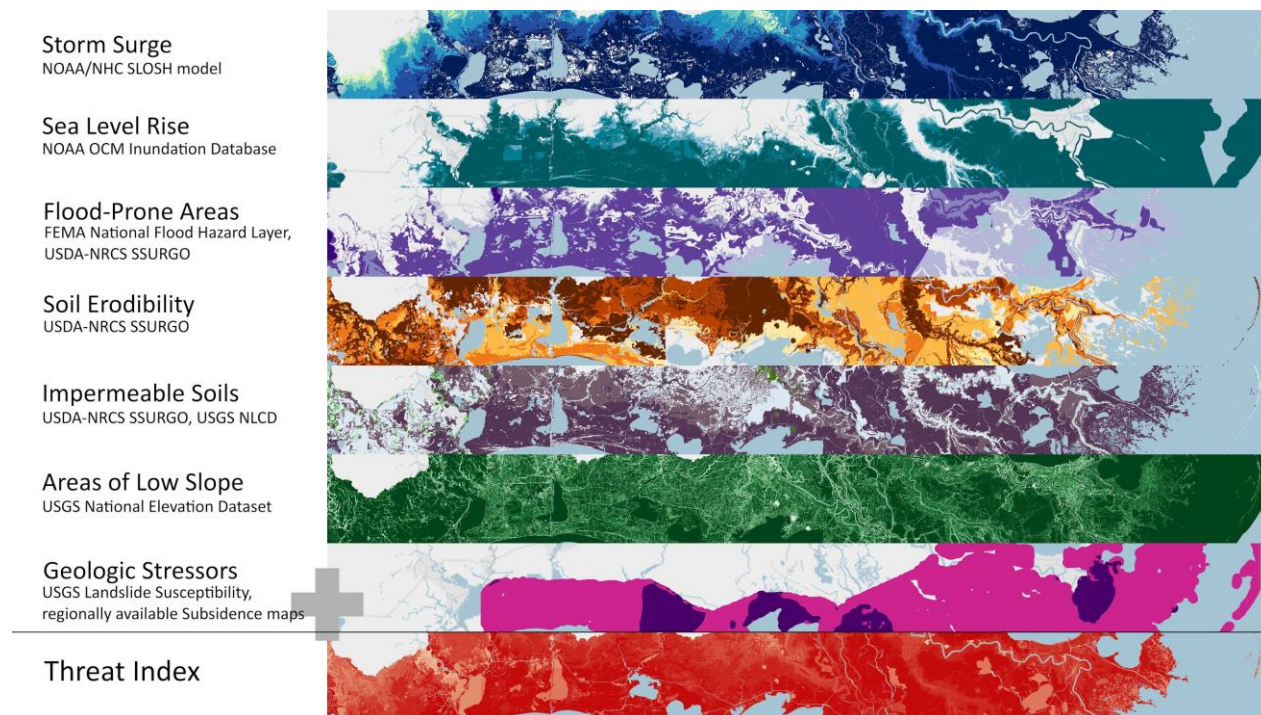
Figure 12. An example of all inputs (listed on the right) used to generate the resulting Threat Index. Darker colors in each input equate to higher rank values. The darkest red in the Threat Index is the highest value.
