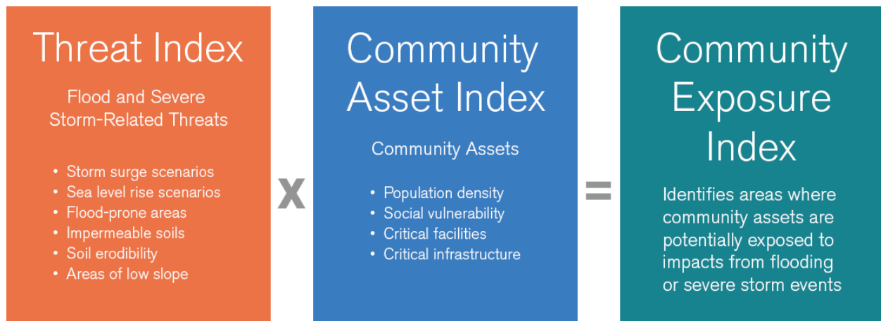
Figure 4. Elements of the Threat and Community Asset Indices used to create the Community Exposure Index.
