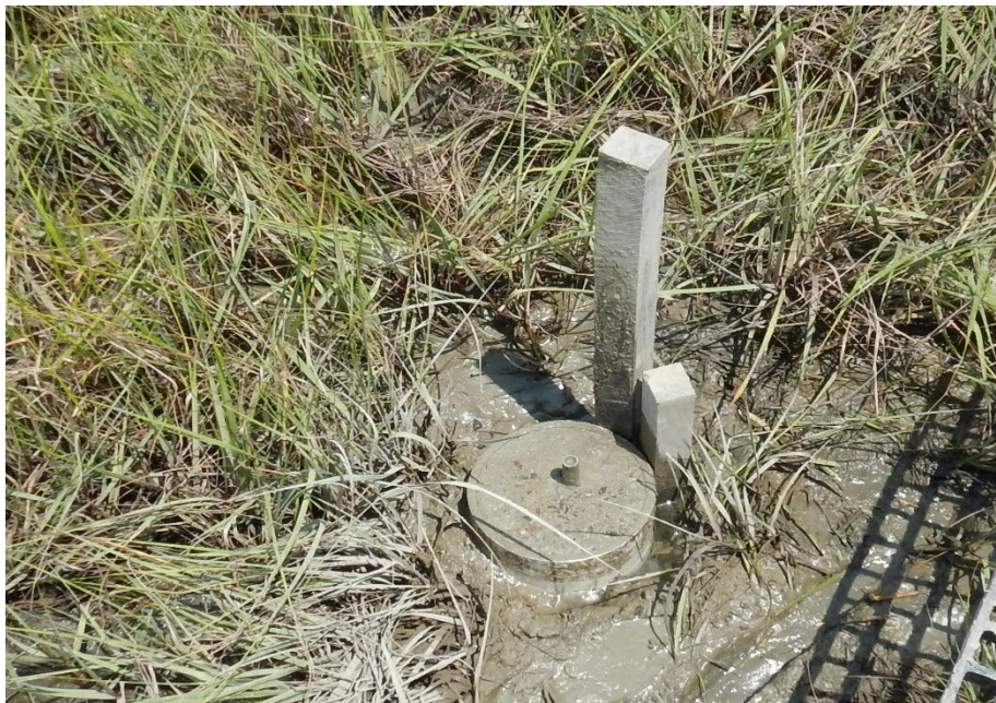
Figure 12: Rod with PVC "collar" filled with cement
